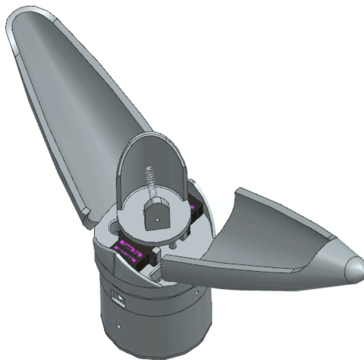
Figure 4: Nose-cone deployment mechanism (open) — CAD
